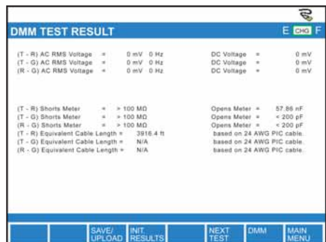
Measure AC / DC Voltage, Resistance, and Capacitance
