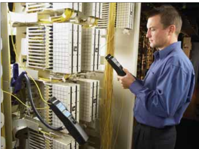
EXFO offers a flexible clip-on arm to enable single-person use of the LFD-300 and TG-300 combo.
